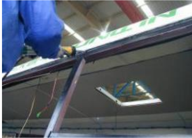
Fig. Injecting glue into the gaps
