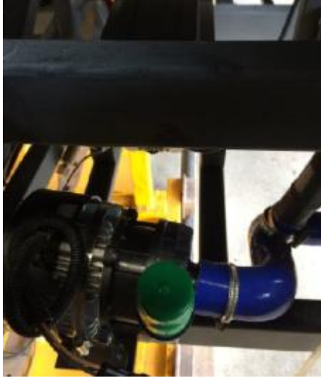
Fig. Water pump inlet hose
