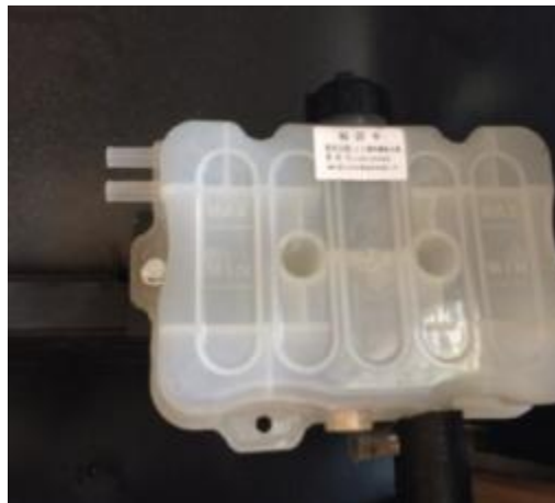
Fig. Installation position of water tank
