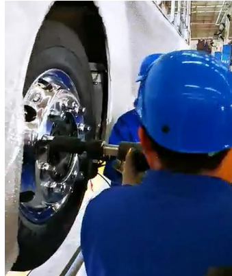
Fig. Tire Installation
