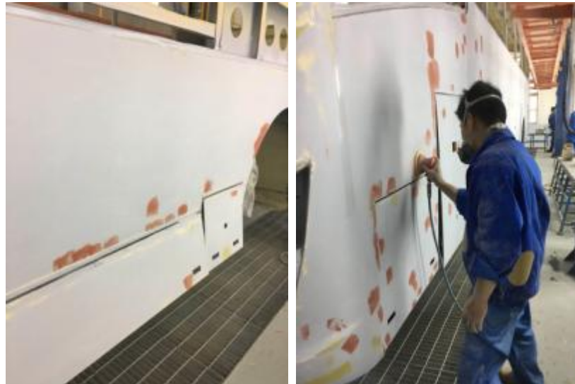
Fig. Filling the surface of the entire vehicle
