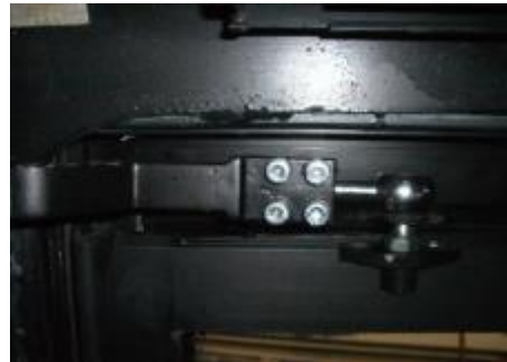
Adjusting the left and right upper control arms
