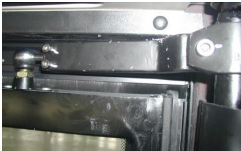
Fig. Mark for bolt tightening
