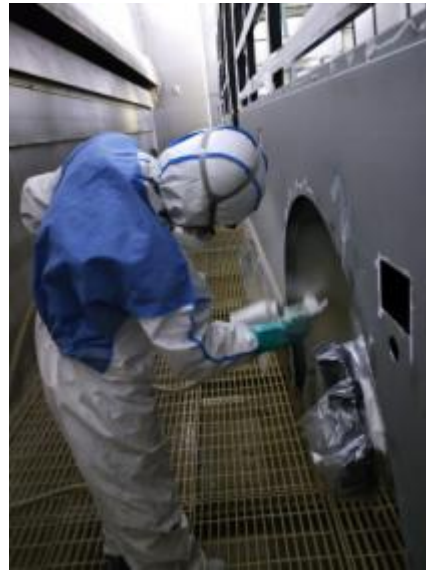
Fig. 7-2 Wheelhouse primer spraying
