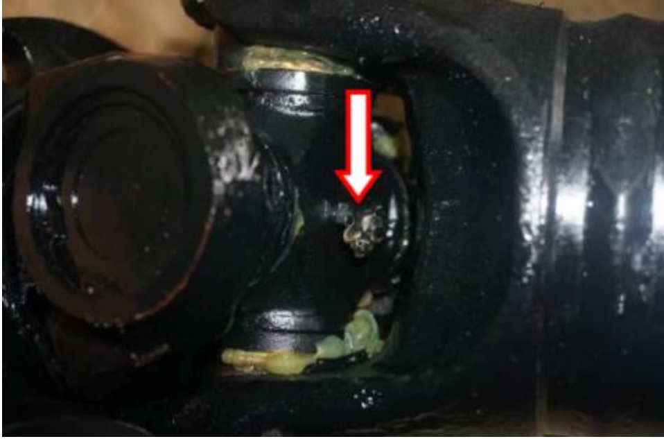
Fig. Location of oil injection port
